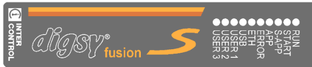
Figure 3-11: digsy ® fusion S (T1/T2/T3) central label with LED indicators
