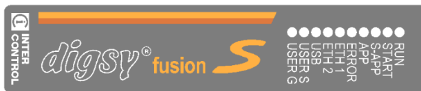
Figure 3-12: digsy ® fusion S-P(L) central label with LED indicators
